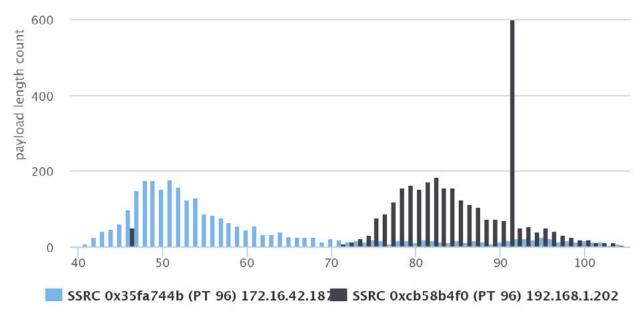
On average, the packets sent by the iOS app (blue) are about 30 bytes smaller, the size distribution is shifted to the left compared to the Chrome (black) one. This is probably the result of a lower target bitrate setting. The big spike at a payload size of 91 bytes is caused by a long period of time where just this packet size is sent by Chrome.
