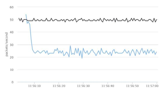
Compared with other sessions, which used at rate of 50 packets/second, the blue graph of the client using the 3G networks shows a much lower rate of 25 packets per second. And while the received bitrate varies strongly between 10 and 30kbit/s. This seems to be one of the adapations to the different network properties.
